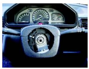
4. With the steering wheel removed, place the hub kit onto the exposed spline on the steering column.
