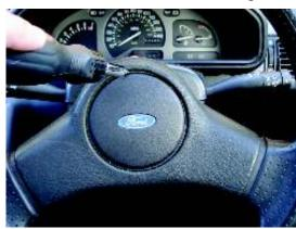
2. Remove the bolt from the steering column. Keep hold of the bolt as it will be replaced later in the process.
