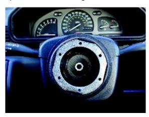
5. Replace the bolt and tighten to secure the hub kit to the steering column.
