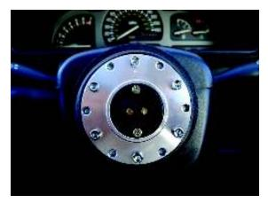
8. Once the rear part of the quick release is secured to the hub kit, replace the front half (it should push into position click and lock.)
