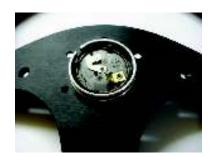
12. Secure the steering wheel to the quick release using the 6 x hub fixing screws.
